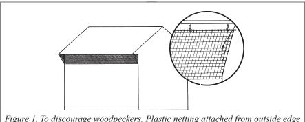
Figure 1. To discourage woodpeckers. Plastic netting attached from outside edge of eave, angled to siding. Insert shows hooks and wooden dowels to attach.
