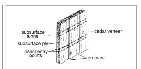
Figure 4. Grooved plywood siding allows insects to burrow their way in.
